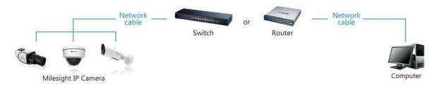
Figure 2-1-2 Connect via a switch or a Router
