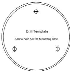
Figure 2-7 Drill Template of Type I Turret Camera
